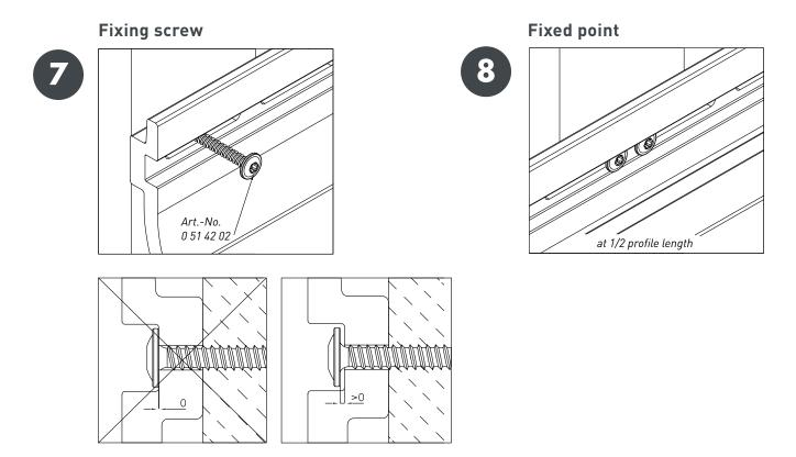
The fastening screws must be centred in the elongated holes and must not be tightened to tension.
