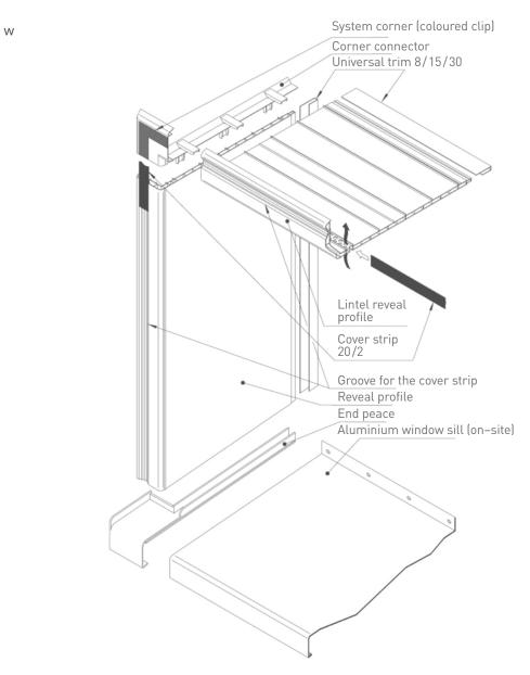
For ventilation of the facade surface below the window sill, a gap of at least 20 mm must be left between the upper edge of the vinyClassic profile and the lower edge of the window sill. To avoid soiling of the facade surface, we recommend a window sill projection of 3 – 4 cm and the installation of window sill end pieces (Art.-No. 0 63 60 \_\_\_).
