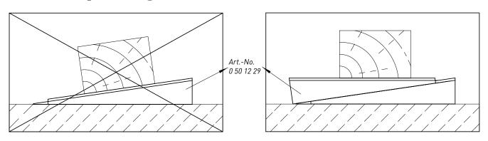
Unevenness of a house wall can be compensated with mounting wedges. Twisting of the battens should be avoided. If facade profiles are installed on twisted or uneven substructures, warping can occur.
