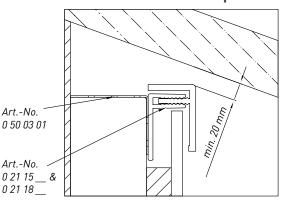
The accessory profiles are also subject to thermal expansion in the event of temperature increases. It is essential to make sure that there is sufficient space for expansion at the profile ends to other fixed components. The upper parts of vertically mounted 2-part accessory profiles must be fixed against slipping in the upper area, e.g. with mounting adhesive or screws.
